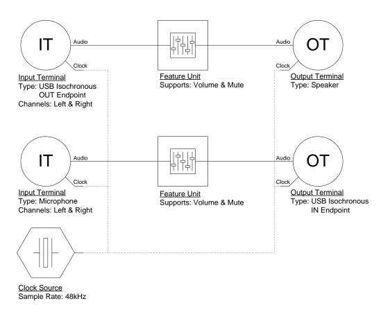
More complex audio devices are created by connecting multiple Unit entities together to describe the Device's capabilities. For more information about the available Unit and Terminal entities, and how they are used please refer to the USB Audio Class Device v2.0 specification.
